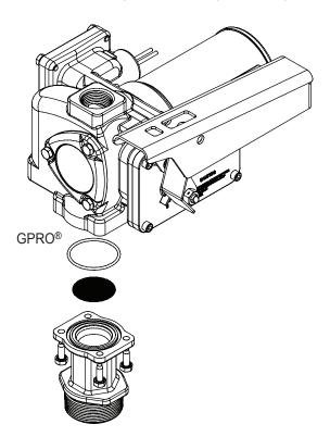
Turn the pump off and disconnect from power. Remove and clean the strainer with a soft-bristled brush and solvent. If the strainer is very dirty, compressed air may be used. If damaged, replace the strainer.
