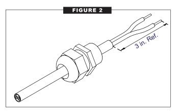
Insert the power cord through the 3/4 inch NPT connection on the side of the electrical box.
